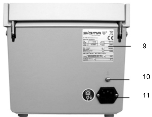
Fig. 5.2: Rear view of the centrifuge
